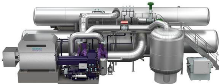
Figure 1: Heat pump system SHP-C600 producing up to 40MW of heat for district heating systems. Including evaporator, condenser with sub-cooler, expansion valves, flash tank, and two-stage compressor.
