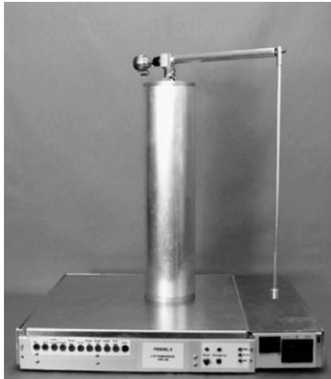
**Figure 7.1** The Furuta pendulum.
